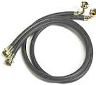
OM8FX90 8' inlet hose 3/4 x 90° - 96-inch long black EPDM automatic washing machine inlet hose with 90° elbow. - OEM grade. - Plated Steel connections.
